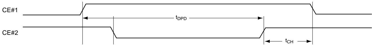
Figure 33. Deep Power-down Timing
